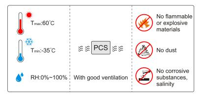
Figure 3-3 Installation environment requirements
