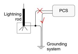
Figure 3-14 Grounding diagram
