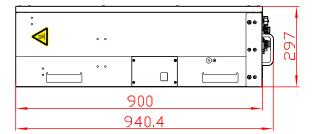
Figure 2-8 Size (unit: mm)
