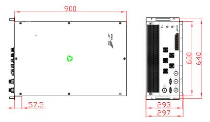
Figure 3-12 Installation size of side stand mounting
