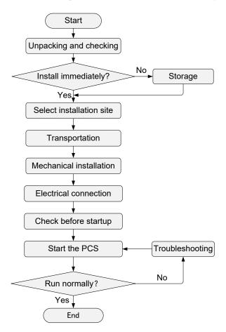
Figure 3-1 Installation process
