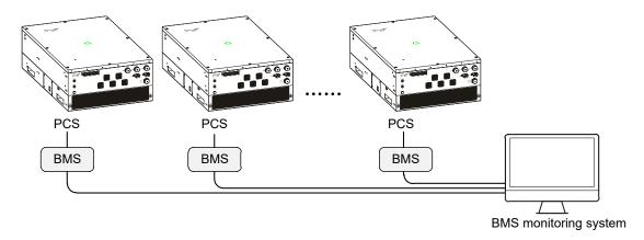
Figure 2-12 Communication with BMS (multiple PCSs)
