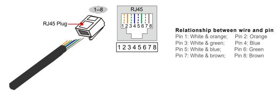
Figure 3-29 Relationship between Ethernet communication wire and pin
