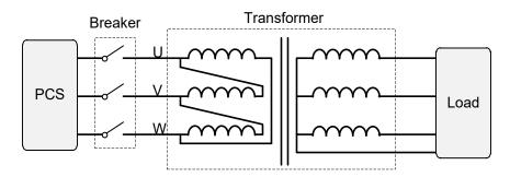
Figure 3-16 Connection diagram (off-grid mode)
