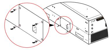
Figure 6-1 Loosen the screws of fan cover
