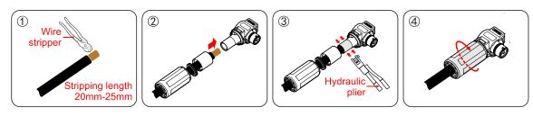
Figure 3-17 Crimp AC cables
