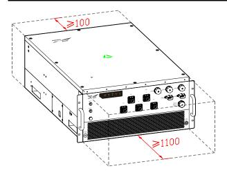
Figure 3-4 Installation Space (unit: mm)
