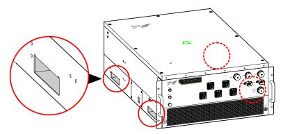
Figure 3-5 Groove position
