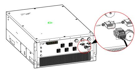
Figure 3-26 COM connection diagram
