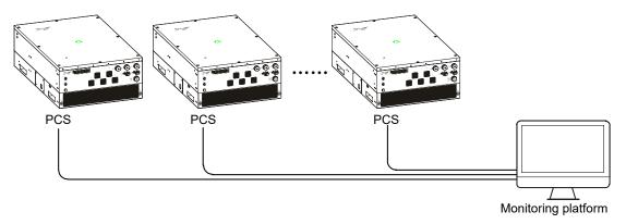
Figure 2-10 Monitoring via Ethernet (multiple PCSs)
