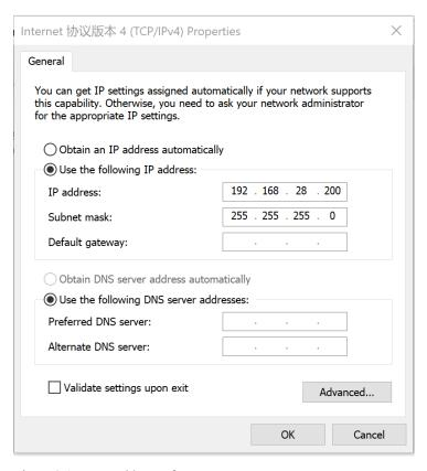
Figure 4-1 Set IP address of computer
