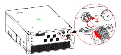
Figure 3-31 ETH port connection diagram
