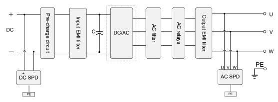
Figure 2-9 Working principle diagram
