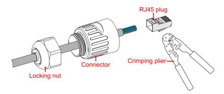
Figure 3-28 Crimping diagram of Ethernet communication wire
