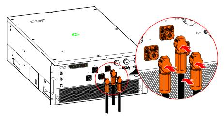
Figure 3-18 AC connection diagram
