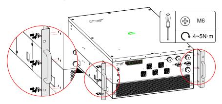
Figure 3-6 Install the fasten parts
