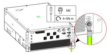
Figure 3-13 Grounding connection diagram
